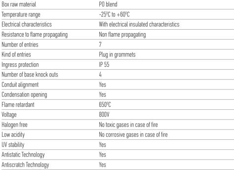
\* Cover plate and plug in seals are made of PE
